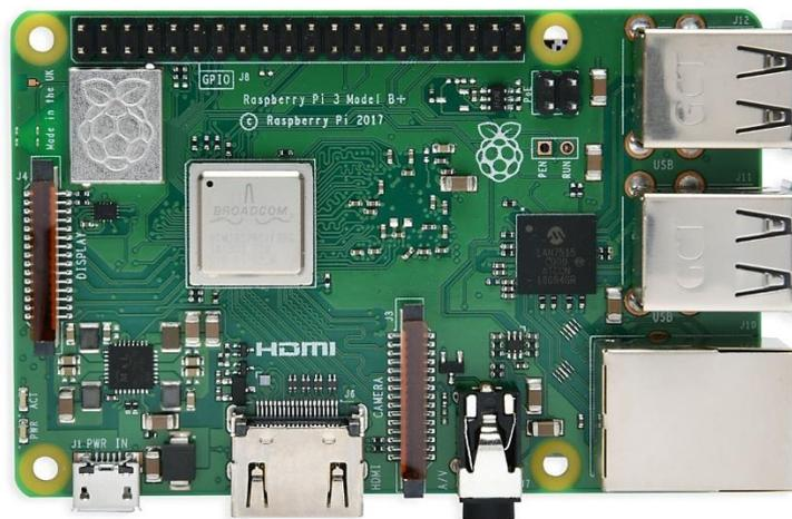
**Gambar 2.2 Raspberry Pi Model 3 B+**
