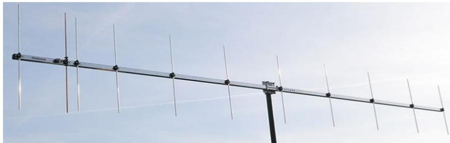
**Gambar 2.10 Antena Yagi 162 MHz Marine Automatic Identification**
