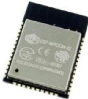
**Gambar 2.4** Chip Mikrokontroler ESP32 (Nodemcu. 2020)
