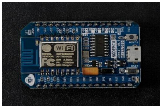
Gambar 2.3 NodeMCU generasi pertama / board V.0.9 ( v1)[12]
