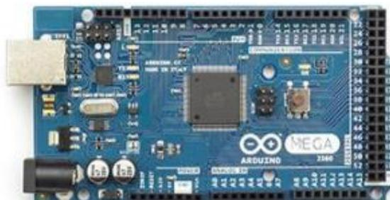
Gambar 2.5. Arduino Mega 2560 [12]
