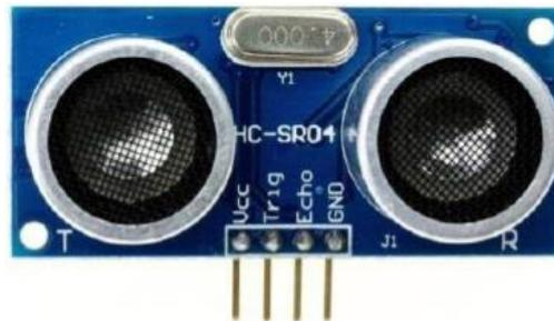
Gambar 2.2. Sensor Ultrasonik HC-SR04[8]
