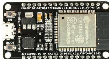
**Gambar 2.2** NodeMCU ESP32
