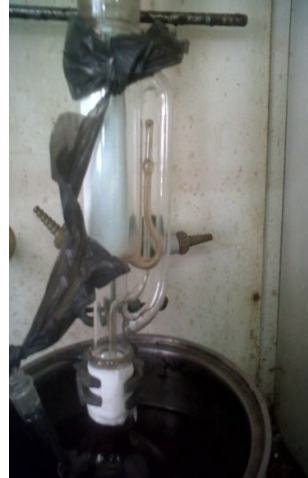
(f). Proses Ekstraksi Soxhlet
