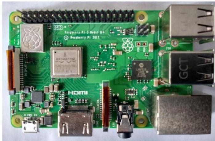
**Gambar 2.16** Front Side Raspberry Pi 3 Model B+
