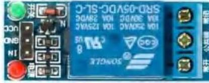
**Gambar 2.7 Modul Relay 1 Channel [6]**
