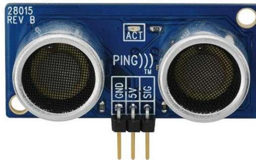
Gambar 2.13 Sensor Ultrasonik PING[22]
