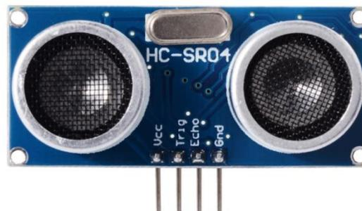
Gambar 2.14 Sensor Ultrasonik[21]
