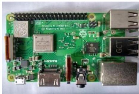
**Gambar 2.2** Bagian Depan *Raspberry pi 3 Model B+*
