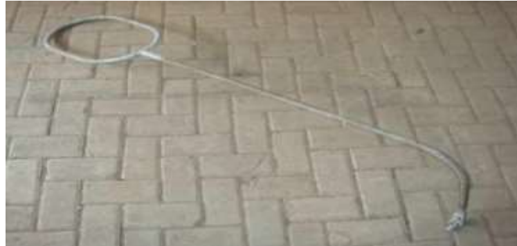
Gambar 2.27 Arcing horn sisi tower
