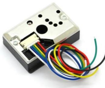
Gambar 2.9 Sensor GP2Y1010AU0F [27]
