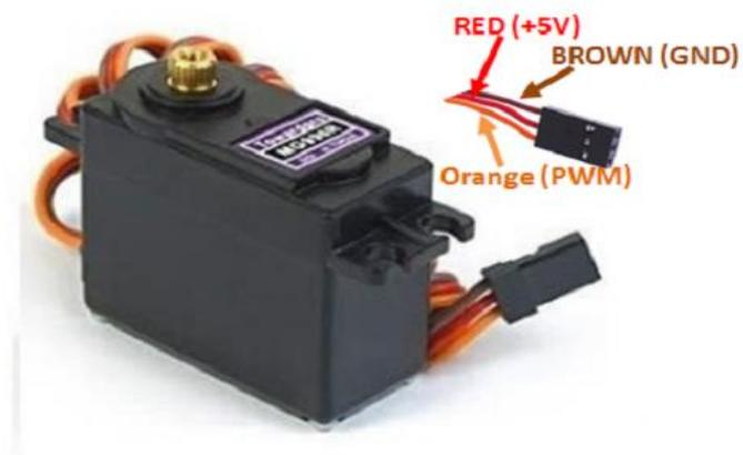
**Gambar 2.8 Motor Servo (Tower Pro MG996R) [6]**
