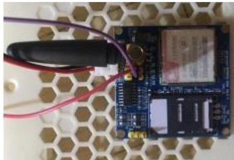
Gambar 2.6 Modul GSM SIM900A[16]
