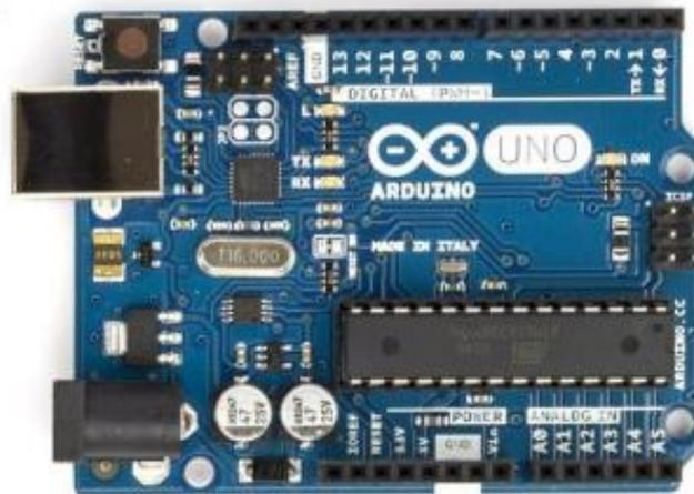
**Gambar 2.4** Board Arduino Uno
