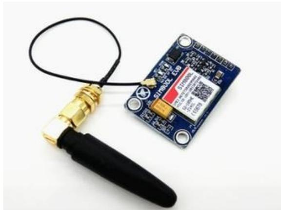
**Gambar 2.8** Modul GSM SIM8001 V.2
