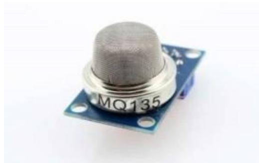
**Gambar 2.2** Sensor Asap MQ-135
