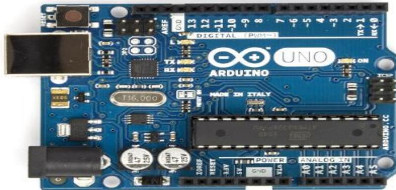
Gambar 2.5 Arduino UNO R3 ATmega328
