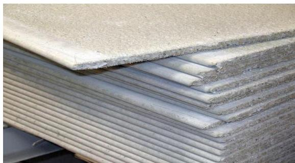
Gambar 2.15 *Glassfiber Reinforced Cement Board (GRC)*
