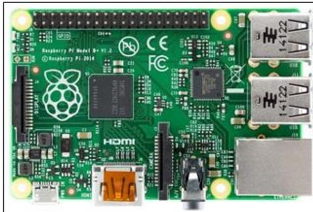
**Gambar 2.3.**Raspberry Pi 1 Model B+<sup>[5]</sup>
