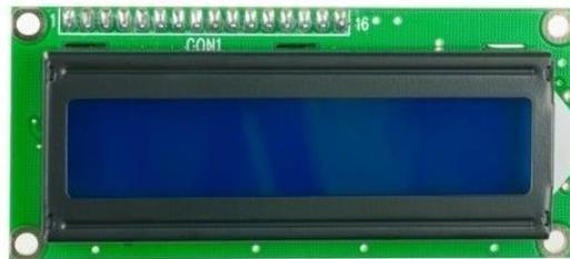
**Gambar 2.8** Liquid Crystal Display 16x2
