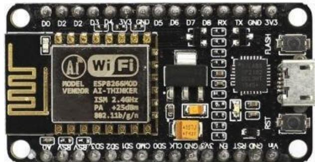
**Gambar 2.1** NodeMCU ESP 8266 [5]
