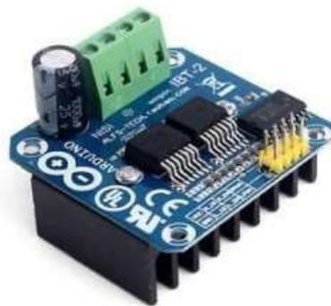
**Gambar 2.18** BTS7960 Driver 43A H-Bridge Drive
