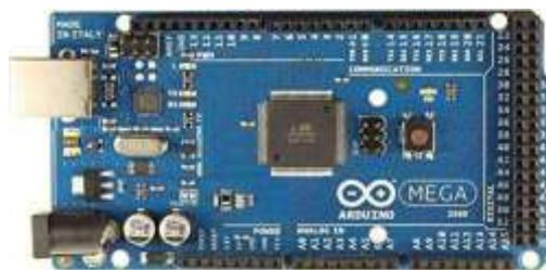
**Gambar 2.6 Arduino Mega 2560**
