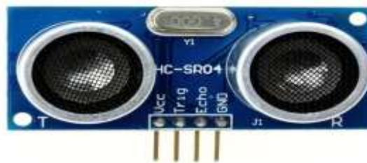
**Gambar 2.4** Sensor ultrasonik HC-SR04
