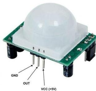
**Gambar 2.7 Pin Sensor PIR**
