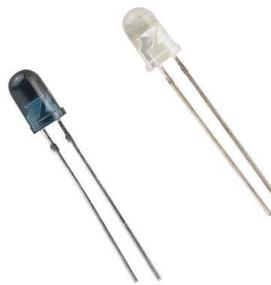
**Gambar 2.17** Led Infrared
