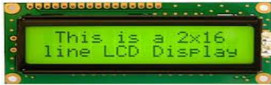
Gambar 2. 16 LCD (*Liquid Crystal Display*)
