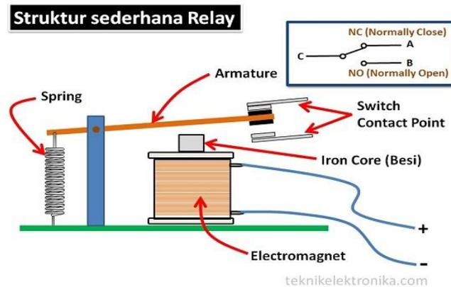
**Gambar 2.2 Bagian-Bagian Relay**
