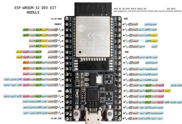
**Gambar 2.5 Pin Out NodeMCU**
