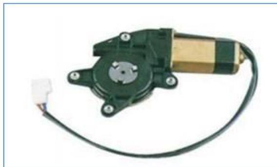
**Gambar 2.17 . Motor DC Power Window**
