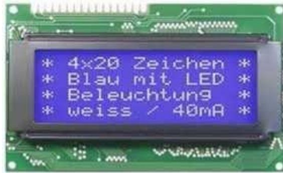
**Gambar 2.20** LCD 4x20
