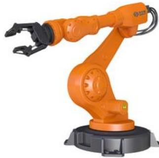
**Gambar 2.2 Manipulator Robot**
