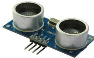
**Gambar 2.9** Sensor Jarak Ultrasonik
