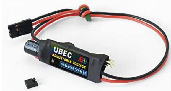
**Gambar 2. 12** UBEC (*Universal Battery Elimination Circuit*)
