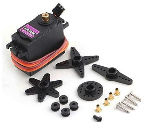
**Gambar 2. 11** Motor servo S996R
