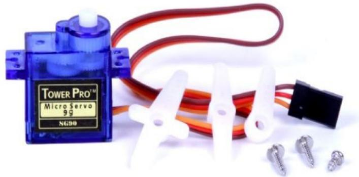
**Gambar 2.4 Motor Servo Sg90**
