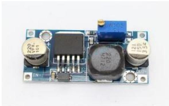
**Gambar 2.8. Modul IC LM2596 DC-DC Step Down Voltage Regulator**
