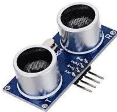
**Gambar 2. 7** Sensor Jarak HC-SR04
