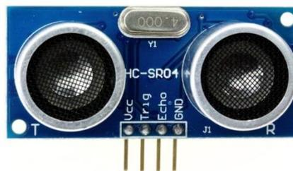
**Gambar 2.2** Sensor Ultrasonik HCR-04
