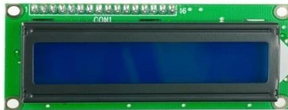
**Gambar 2.3** *Liquid Crystal Display 16x2*
