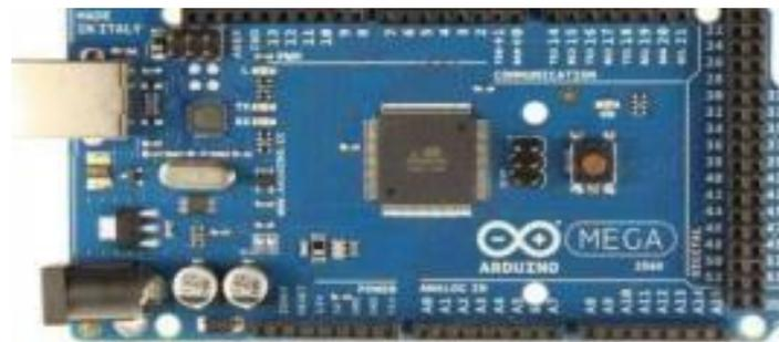
**Gambar 2.7** Arduino Mega 2560
