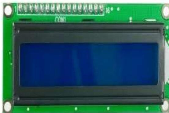
**Gambar 2.10** Liquid Crystal Display 2x16
