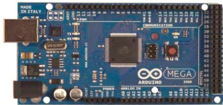
**Gambar 2.11** Arduino Mega 2560
