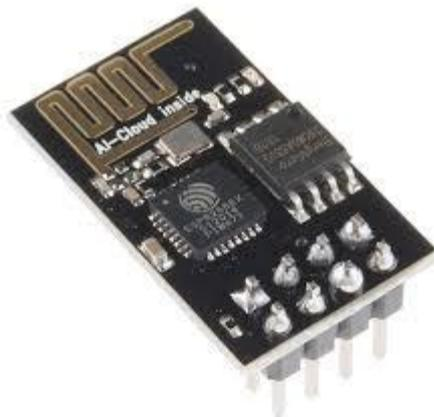
**Gambar 2.8** *module ESP8266 ESP-01*
