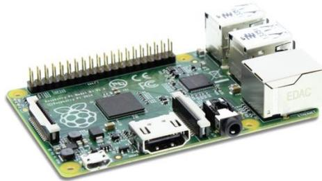
**Gambar 2.4** Raspberry Pi Model B+
