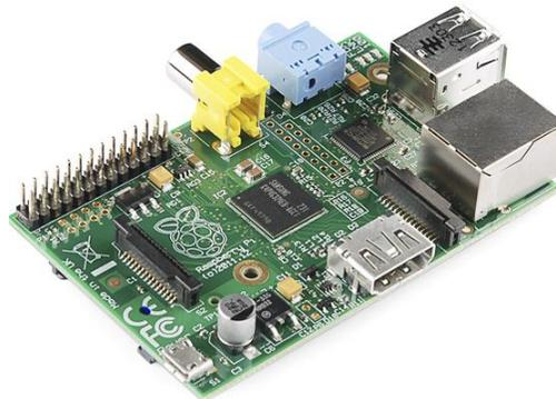
**Gambar 2.3** Raspberry Pi Model B
