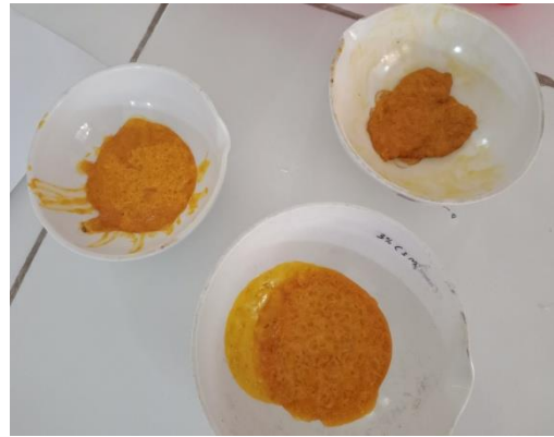
Gambar 34. Proses uji padatan total cat lateks
