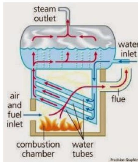
**Gambar 2.2** Water Tube Boiler
