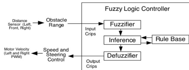
Figure 2. Design fuzzy logic controller
