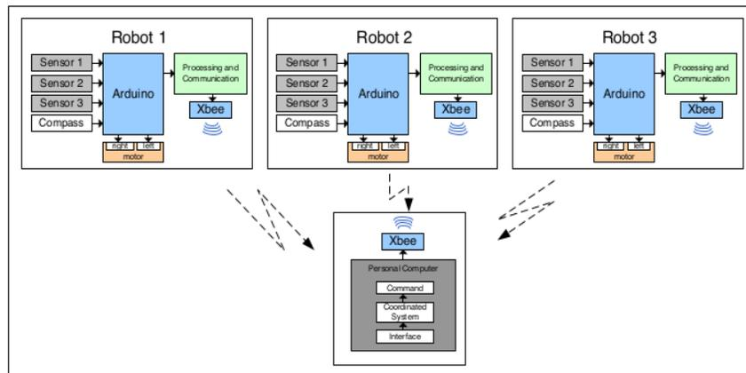
Figure 1. Block diagram control of swarm robot coordination
