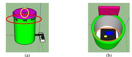
FIGURE 2. Garbage bin proposed in this research (a) ultrasonic sensors placement (b) Component Module placement
