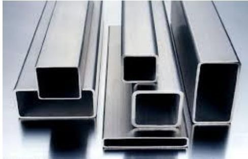
Gambar 2.5 Besi Hollow (Sumber: besibesihollow.blogspot.com )
