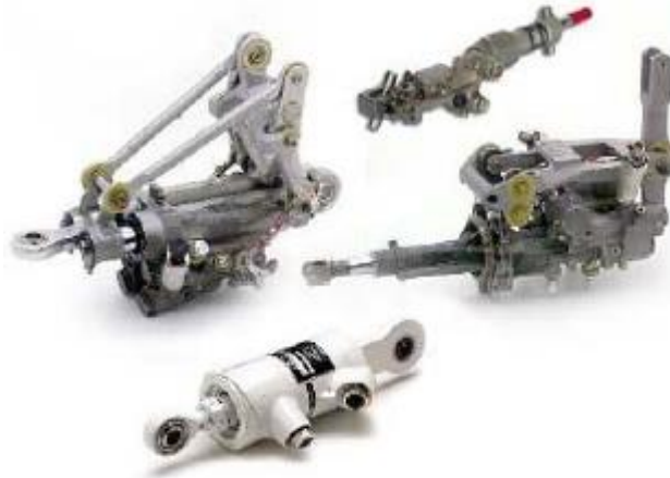
Gambar 2.10 Actuator Hidrolik (Module 10 Aircraft System)
