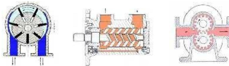
Gambar 2.6 Pompa Kipas, Pompa *Screw*, Pompa Roda Gigi
