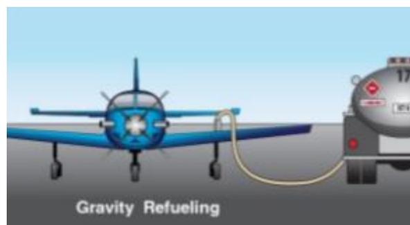
Gambar 2.1 *Gravity Refueling*
