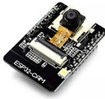
**Gambar 2.12** ESP32-Cam
