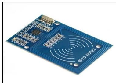
**Gambar 2.1** *Radio Frequency Identification (RFID)*
