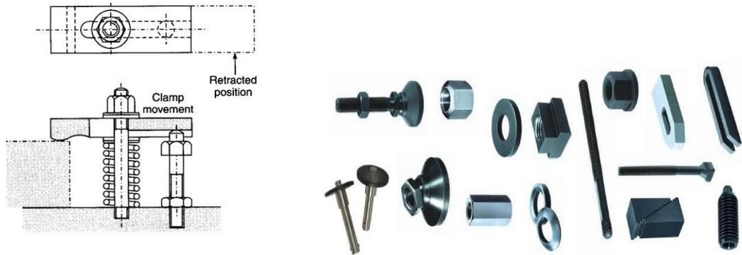
Gambar 2. 10 *Slotted Plate Clamp*
