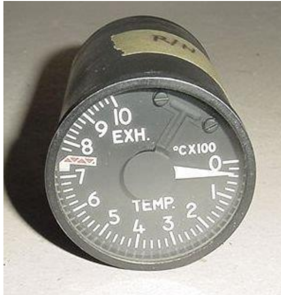
Gambar 2.5 Exhaust Gas Temperature Indicator tipe moving coil [6]
