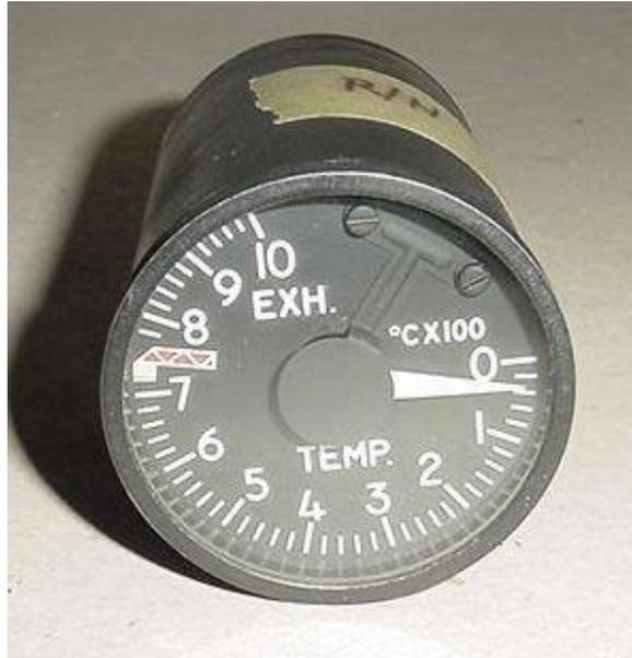
**Gambar 2.5** Exhaust Gas Temperature Indicator tipe moving coil [6]
