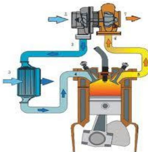
Gambar 2.8 Cara Kerja Turbocharger [7]
