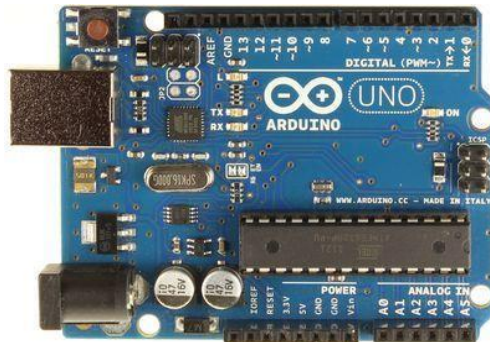
Gambar 2.1 Arduino UNO R3 [3]
